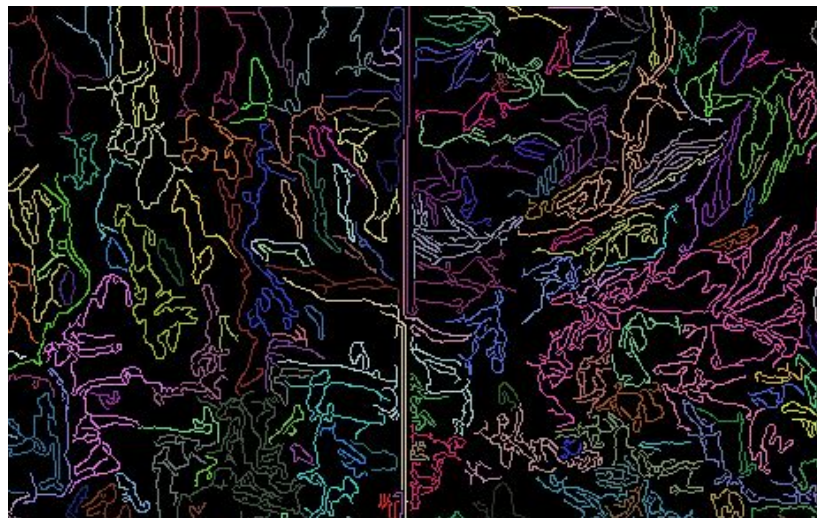
Figure 4: Close up of colorized ridges and valleys in the ranch. Each pixel in this image represents a distance of 30 meters. Note the seam caused by GIS stitching in the center of the image.
